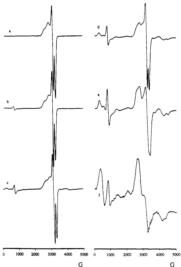
Figure 10. Thermal variation of the EPR spectra of [\text{Cu}_4(\text{H}_2\text{O})_2(\text{P}_2\text{W}_{15}\text{O}_{56})_2]^{16-} (II): (a) T = 5.5 K; (b) T = 17 K; (c) T = 28 K; (d) T = 50 K; (e) T = 130 K; (f) T = 300 K.
