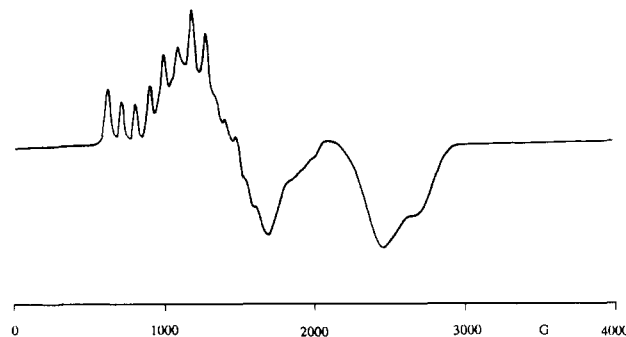
Figure 6. EPR spectra of the 5% cobalt-doped Keggin derivative Zn compound at 4.2 K, \{[Zn,Co]_4(H_2O)_2(PW_9O_{34})_2\}^{10-} , showing the range of g values for the cobalt compounds.
